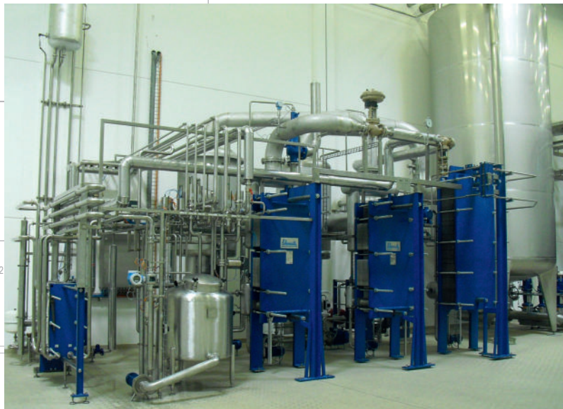
2-stage SIGMASTAR® 90V Evaporating Plant plant extracts - evaporating capacity 3,000 kg/h
