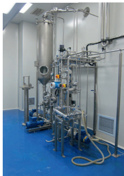
1-stage SIGMAVAP Evaporating Plant pharmaceutical products - evaporating capacity 500 kg/h (ATEX-version)
