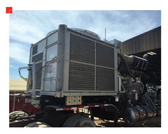
When it comes time to replace the traditional horizontal cooling module on a frac track, consider a compact cube unit. The innovative cube design offers many advantages over the standard, horizontal module, including higher efficiency, better reliability, easy-access cleaning, and a longer lifecycle.
