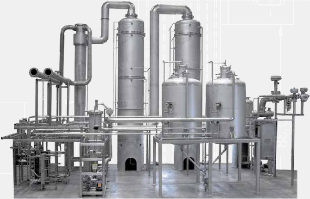
Dealcoholization plant for beer - 100 hl/h beer - preassembled in the workshop
