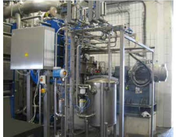
SIGMASTAR 90V MVR – Evaporating capacity: 2.000 kg/h
