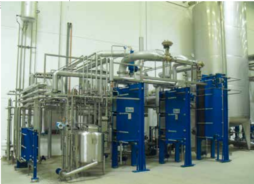
2-stage SIGMASTAR® 90V Evaporating Plant plant extracts - evaporating capacity 3,000 kg/h
