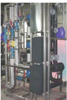
Compact reactor heating-cooling module
